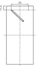
2 Drill holes on the marks and insert wall plugs. Screw the wall mount onto the wall. Plugs and screws not included.
