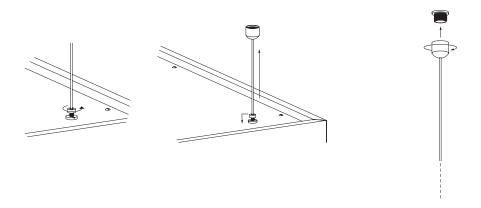
Once all four top caps have been screwed onto the ceiling, press down the wirelock once more to adjust the length of the wire. The wire can be pushed up and down.
